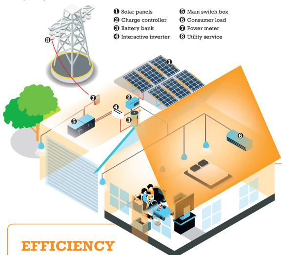
It is important to choose the right components for the most effective use of solar PV systems. A PV module
